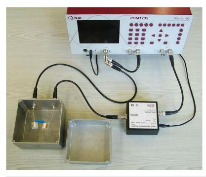
Accessory for use with the PSM1700 or PSM1735 Frequency Response Analyzers for high impedance measurement.
