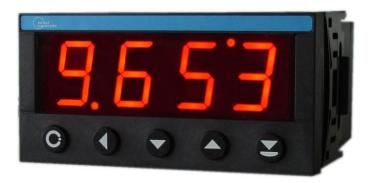
*Tare* can be activated with the keyboard and force the display to zero. The Tare remains memorized also when the instrument is switched-off from the supply. The Tare can be canceled at any time and the display returns to follow the original input signal.
