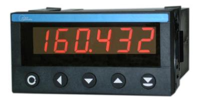
Model OC7056A is a six digit programmable controller with 200000 true increments. They can be scaled within the full display range 0-999999. The controller is mainly designed for process signals such as 0/4-20mA, 20mV to 300V DC or true RMS, strain gauges, Pt-100, Pt-200, Thermistor, Resistors and DIN-Thermocouples.
