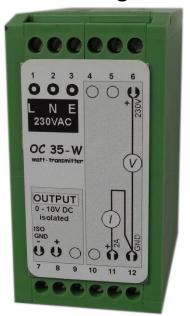
**OC35-W** are transmitters for true R.M.S. power measurement. Voltages up to 250V and currents to 5A can be directly connected. Larger currents can be connected via current transformers or shunts. The output signal is isolated by 250V R.M.S. from the input and the supply.
