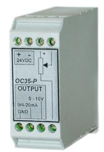
**OC35P-DAY** has very high accuracy and stability. Potentiometric sensors between  $1k\Omega$  and  $100k\Omega$  can be connected. For rotative sensors the output signal can be calibrated in degrees e.g.  $0\dots345\,^{\circ}=4$  - 20mA.
