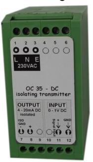
**OC35-DCP** are transmitters for potentiometric sensors. They convert the displacement or the angle of the potentiometer into 4-20mA, 0-10V or 0-3.60V analogue output. They are supplied from the mains or from DC voltage. The connected potentiometers are supplied from internal precision voltage reference. The analogue outputs can be ordered isolated or non-isolated.
