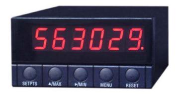
**Model INF8-EnDat** is a 6 digit counter for a direct connection to EnDat serial interface of Absolute Coded Resolvers. The counter is front programmable with the keyboard and uses a high speed microcontroller. Standard features are multiplication and division of the display readings, preset and reset, four set points, two analog outputs and two serial data ports.
