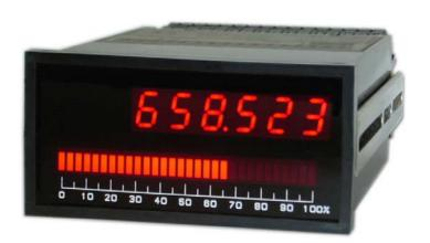
Model OC7167 is a programmable counter with a digital display and a bargraph. The digital display has six digits. During the measurement, five digits are used with a maximum readout of 99999. All six digits are activated in programming mode. The bargraph has 30 red LEDs.
