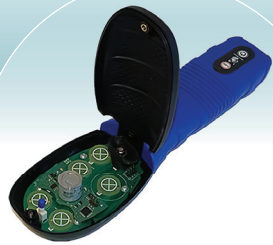
DSII-3 Probe with *C/*F, %RH sensors (1 more sensor can be added)
