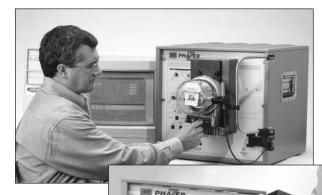
A Universal A-base adapter can easily be installed on a PHAZER Model J120 to facilitate the efficiency of testing both S-base and A-base watthour meters.
