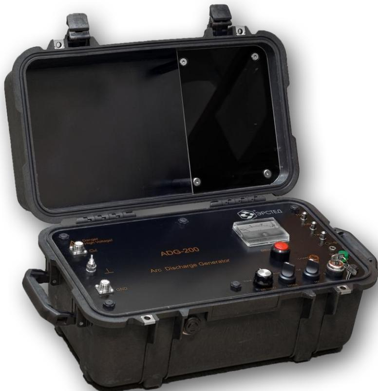
Arc Discharge Generator ADG-200-2 is designed to work on the fault location in combination with the TDRs: RI-407 / TDR-107 / TDR-109 and with the third party TDRs (with ARM and ICE methods support), significantly expands their ability to location of high impedance defects which are not localize with low-voltage TDR method.
