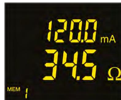
Standard mode: Impedance and leakage current
