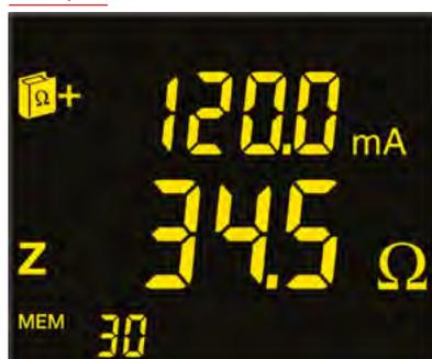
Screen 1: Impedance and leakage current
