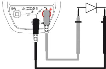
5. Read the junction threshold voltage measurement indicated on the display.
