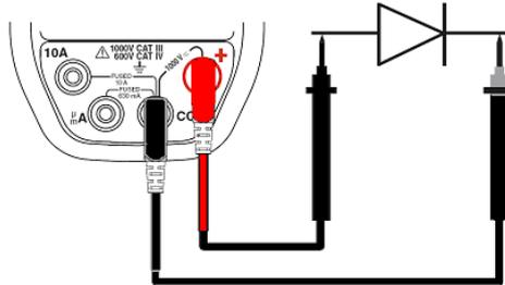
5. Read the junction threshold voltage measurement indicated on the display.
