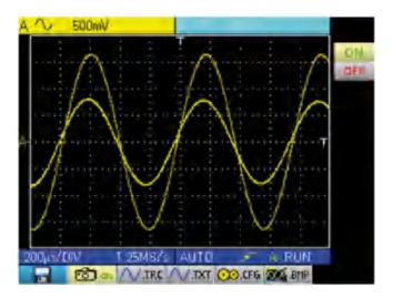
A reference memory is volatile; it is lost when the instrument is powered off, or when the channel or reference is deactivated.
