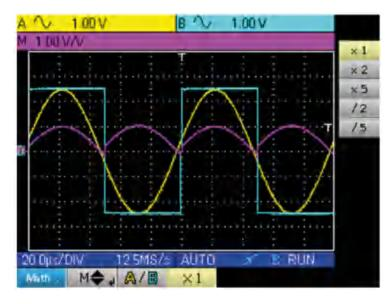
As the positive voltages of signals A and B are equal, the division leads to a positive peak voltage of 1 V/V, and therefore a representation of 1 division on the trace. This can be expanded by choosing factor x 2 or x 5:
