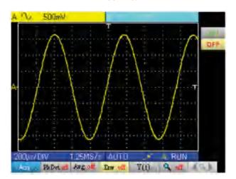
■ with envelope (an acquisition is displayed at each triggering):
