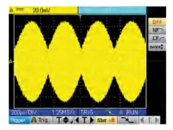
■ with the HF reject filter (the noise is filtered, we trigger on the 1 kHz sine:
