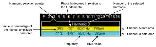
This window displays the specific measurements of the selected harmonic for each channel. The following measurements are displayed:
