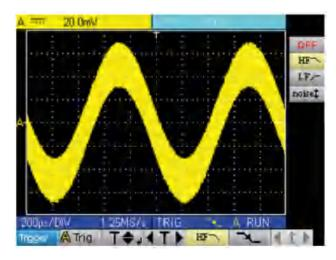
■ with the LF reject filter (the 1 kHz signal is filtered, we trigger on the noise → not effective in this case):
