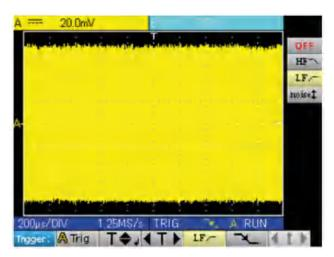
■ with the Noise filter (the trigger hysteresis changes to 3 div., we trigger on the 1 kHz sine):
