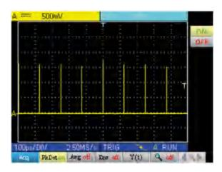
Peak detection deactivates ETS (Equivalent Time Sampling) reconstruction of a repetitive trace. Sampling is real-time for time bases ≤ 2.5 µs/div.
