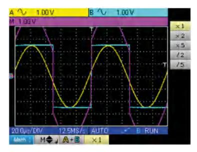
In our example the amplitude of the resulting signal is 10 Vpp. As the sensitivity of channel M is 1 Vpp, it can be seen that the trace overshoots but is contained on the screen by dividing the representation by 2:
