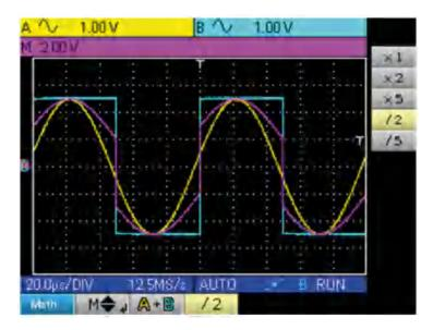
The sensitivity of the M channel becomes 2 V and the amplitude remains at 10 Vpp.
