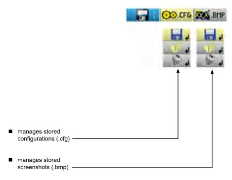
■ The .bmp file can be recovered on a PC using SX-METRO software/ Oscilloscope mode, import memory.
