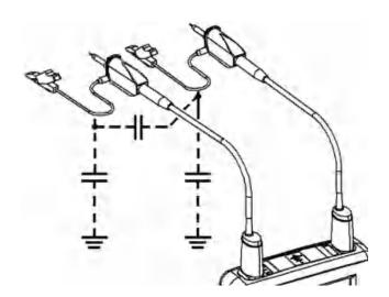
It is imperative, considering the stray capacitances, to correctly connect the reference conductors for each sensor. The conductors should preferably be connected to the cold points to avoid the transmission of noise by the stray capacitance between modes.
