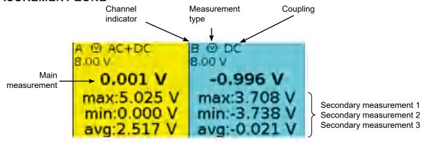
The direct data from channels A and B are displayed in this windows:
