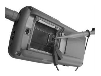
Connect the sensor to be adjusted to the calibration output under the battery housing cover, as shown opposite.
