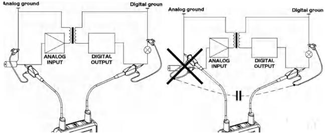
The noise of the digital ground (earth) is sent to the analogue input by the stray capacitance.
