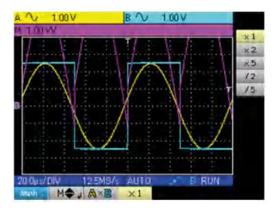
In our example, the peak amplitude of our mathematical function is 2.5 V \* 2.5 V = 6.25 VV. As the channel M sensitivity is 1 VV (with the factor x 1), it can be seen that the trace overshoots and can be corrected by using the /2 coefficient.
