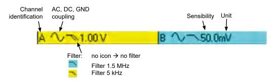
The direct data from channels A and B are displayed in this window:
