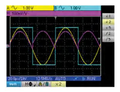
The sensitivity of channel M changes to 500 mV/V and the positive peak amplitude of the trace is 1 V/V.
