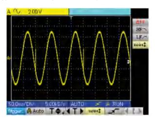
■ LF reject case: (we remove the 10 Hz signal and can trigger on the peak and zoom)
