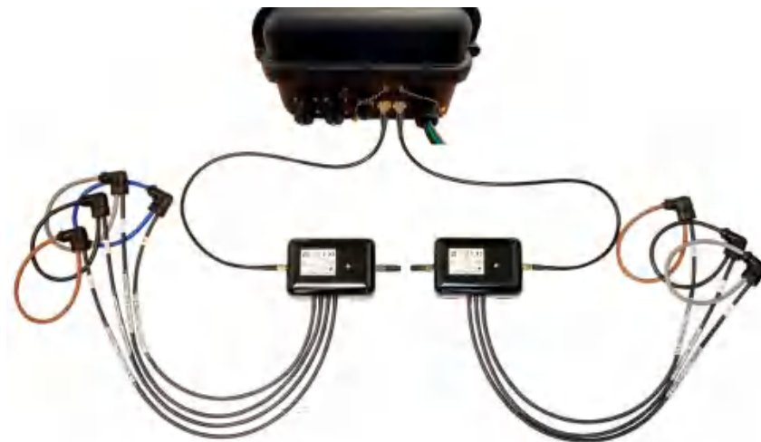
Base unit with connected Current Modules 3PN and 3P
