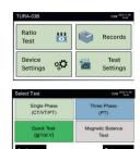
TURA-03 is designed to accurately measure the turns ratio of single-phase and three-phase transformers.
