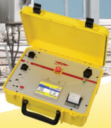
The MARK III 250V is the leader for 3 phase turns ratio measurements. A fully automatic, self-calibrating system with single hook up to transformer, automatic vector group detection and a voltage measurement range up to 250V. A color LCD with back lighting and touch screen increases user comfort. USB interfaces make it easy to store measurements on external
