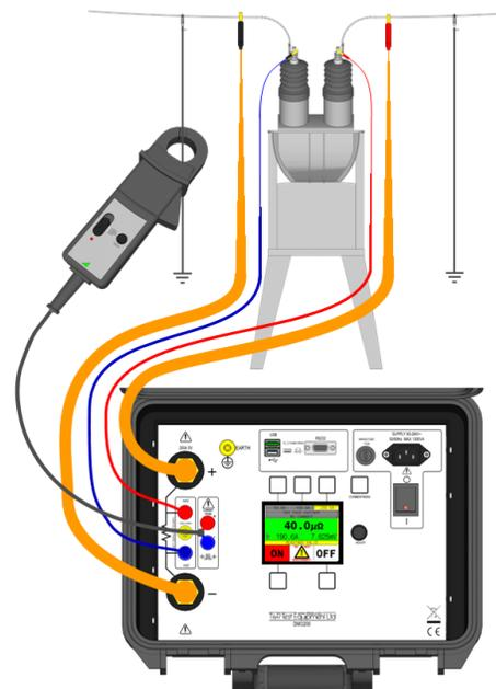
Accurate measurements on circuit breakers, isolators and grounding links with both sides earthed are simple with the optional current clamp. This allows the current flowing through the earthing equipment to be subtracted from the test current.
